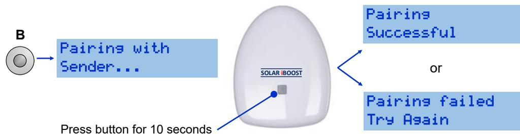
**IMPORTANT!** Do not press the sender button except when performing the pairing process. If it is pressed for more than one second the pairing may be lost and the display shows a 'Lost Signal' message (see Trouble Shooting). To correct, either reset the sender by removing and refitting the batteries or use the above procedure to reset the pairing.
