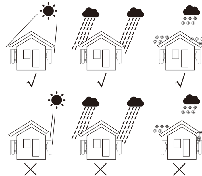
▲ Figure 4.1 Recommended Installation Locations
